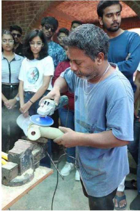
Image 29 Experts using grinder for finishing the joint
